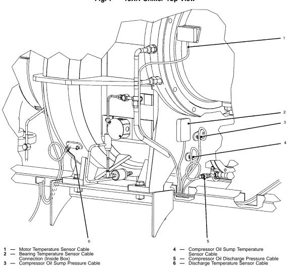
Fig. 8 — Compressor Detail
